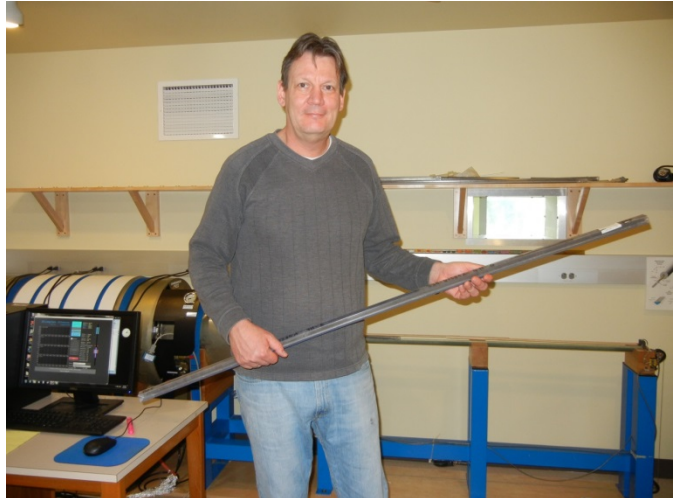
Carl Richter changing a U-channel sample in the shielded room at the University of California at Davis. Pass-through cryogenic magnetometer is in the back.
